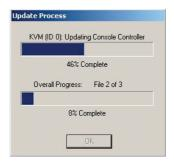
When the update is started, a dialog pops up, displaying the file transfer progress for each sub-device, and for the Switch, as a whole. If multiple devices have been selected, the dialog remains up and repeats the update process for each device. When the update is complete, the "Next" button will become active, allowing the user to complete the update.
